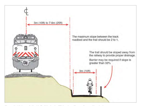
Figure 12: Minimum Rail-with-Trail Setback—Fill Sections (Depending on Situation)
