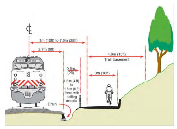
Figure 13: Minimum Rail-with-Trail Setback—Constrained Sections (Depending on Situation)
