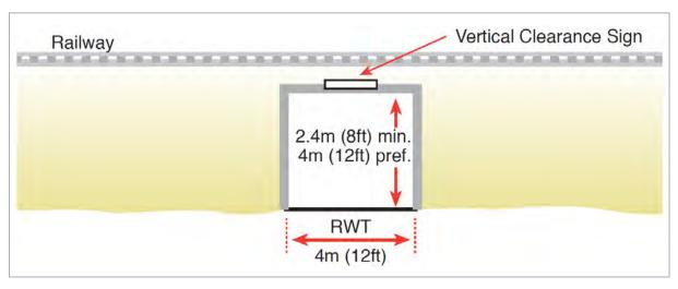
Figure 32: Rail-with-Trail Culvert under Tracks
