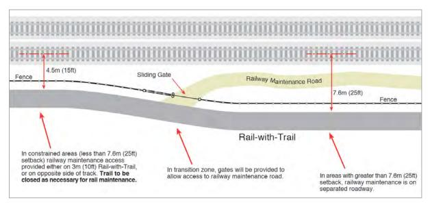
Figure 14: Sample Maintenance Access Transitions
