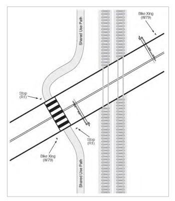
Figure 40: Angled Intersection with Roadway
