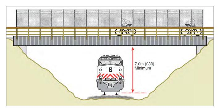
Figure 35: Rail-with-Trail Track Overcrossing (Meets Amtrak-Required Clearance Height for Non-Electrified Track)
