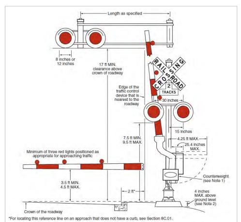
Figure 28: Clearances for Active Traffic Control Devices at Highway-Rail Grade Crossings (MUTCD Fig. 8C-1)
