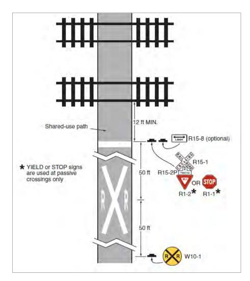
Figure 24: Example of Signing and Markings for a Pathway Grade Crossing (MUTCD Fig. 8D-1)
