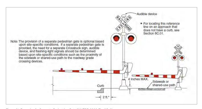
Figure 31: Example of a Separate Pedestrian Gate (MUTCD 2009 Fig. 8C-6)
