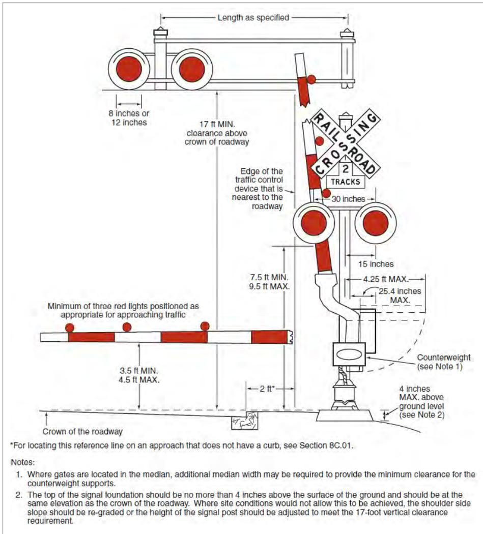
Figure 28: Clearances for Active Traffic Control Devices at Highway-Rail Grade Crossings (MUTCD Fig. 8C-1)
