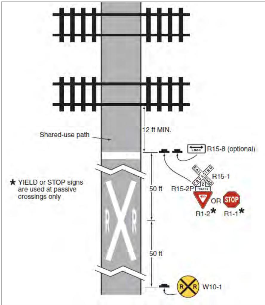
Figure 24: Example of Signage and Markings for a Pathway Grade Crossing (MUTCD Fig. 8D-1)
